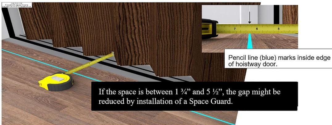
Even if the first measurement indicates that the space between the two elevator doors is less than four inches, take **multiple measurements** at different parts of the elevator car door to determine whether this space exceeds four inches at any point.
